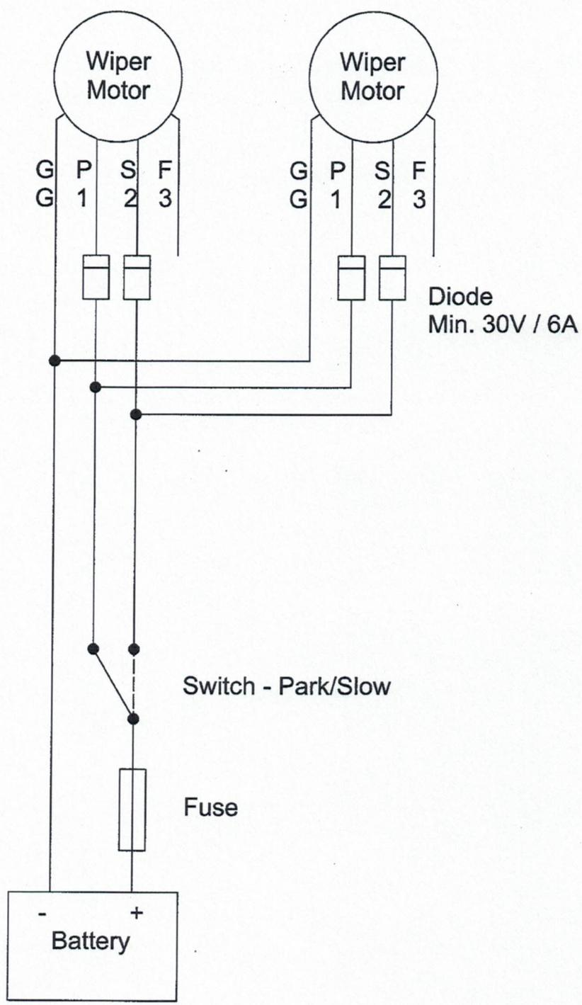
The diodes is needed to make the parking work. If connected without diodes one motor will power - the others and the system will not stop.
